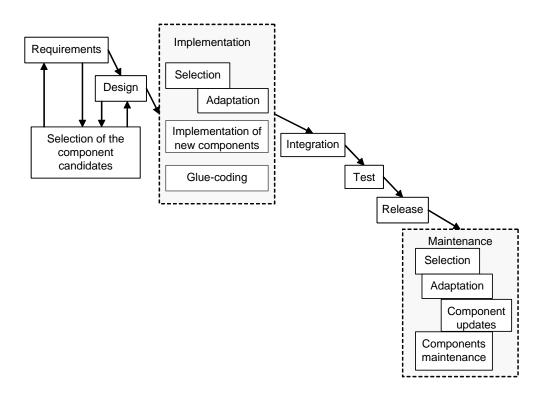
Figure 3: Component-based Waterfall Software product lifecycle
