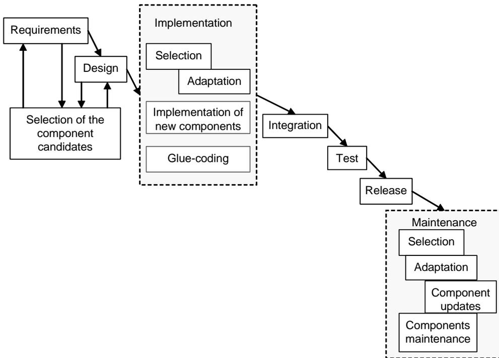
**Figure 3: Component-based Waterfall Software product lifecycle**
